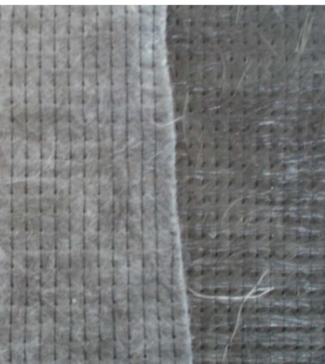
Figure 2: Nonwoven samples made from rCF (a), blend with PA6 (b) and rCF (c) (left to right)
